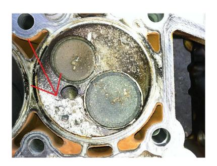
Small metal particles as seen in the picture above will damage the engine. The intake will have these small particles along the wall of the intake. Please make sure you clean your intake.
